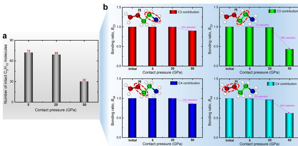
**Fig. 6** Dissociation of C<sub>5</sub>H<sub>10</sub> lubricant. **a** Number of intact C<sub>5</sub>H<sub>10</sub> molecules and **b** bonding ratio for each of the C-C bonds of C<sub>5</sub>H<sub>10</sub> after the friction process, in which only the contribution from the lubricant is considered
