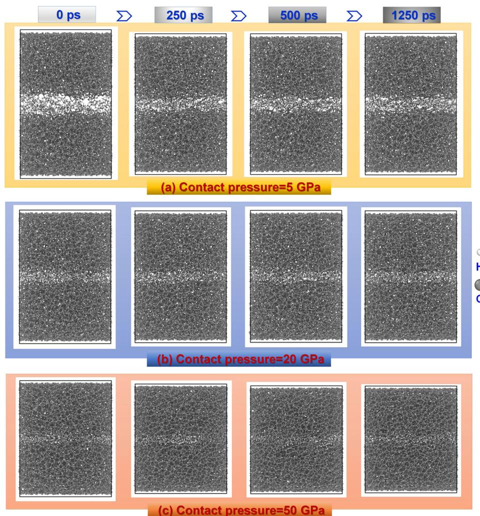
**Fig. 1** Configurations of a-C/C<sub>5</sub>H<sub>10</sub>/a-C friction systems at contact pressures of **a** 5, **b** 20, and **c** 50 GPa
