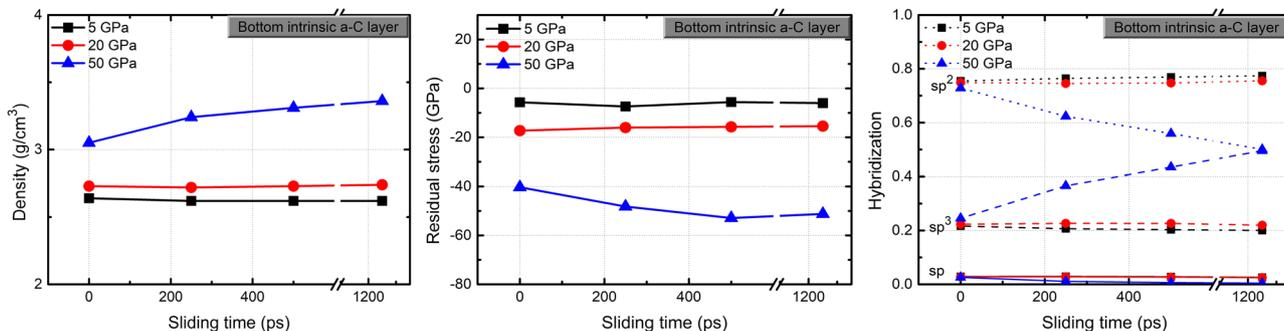
**Fig. 4** Dependence of the density, residual stress, and hybridized structure of the bottom intrinsic a-C layer on sliding time in a-C/ $C_5H_{10}$ /a-C system at different contact pressures
