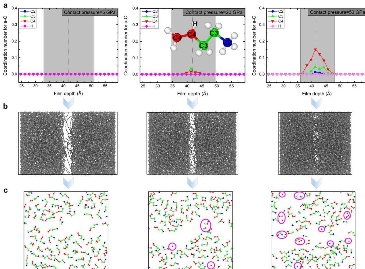
**Fig. 5** Information at the a-C/C<sub>5</sub>H<sub>10</sub> friction interface. **a** Contribution of the C<sub>5</sub>H<sub>10</sub> lubricant to the coordination number of the a-C structure; **b** a-C and **c** C<sub>5</sub>H<sub>10</sub> lubricant structures in the a-C/C<sub>5</sub>H<sub>10</sub>/a-C system after the friction process at different contact pressures
