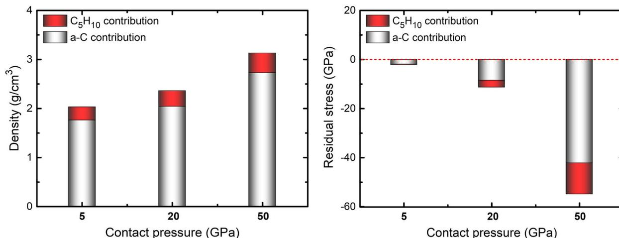
**Fig. 7** Contact pressure dependence of the density and residual stress of the interface contributed by a-C and the C<sub>5</sub>H<sub>10</sub> lubricant, respectively, after the friction process
