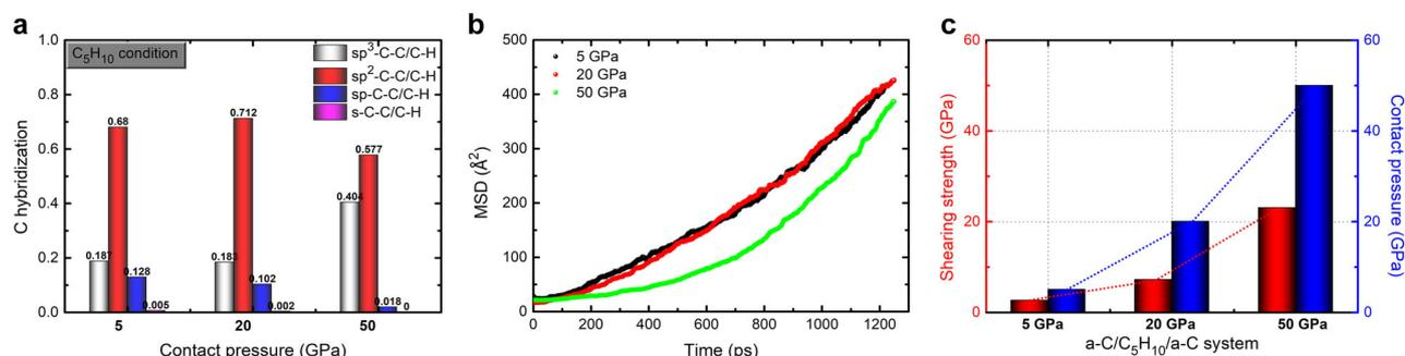
**Fig. 8** Evolution of the interfacial structure with contact pressure. **a** Hybridized structure of the C atoms at the interface as a function of contact pressure after the friction process. **b** MSD of the C<sub>5</sub>H<sub>10</sub> molecules in the a-C/C<sub>5</sub>H<sub>10</sub>/a-C systems. **c** Shearing strength as a function of contact pressure
