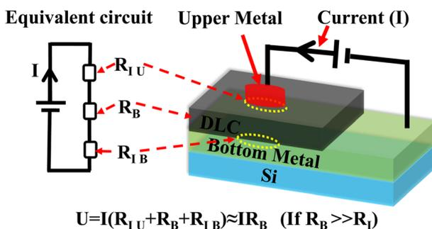
FIG. 4. Equivalent circuit diagram of the MSM device.
