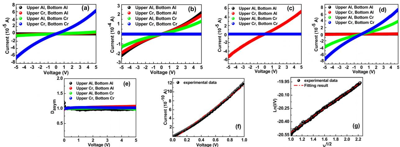
FIG. 2. The I-V curves of MSM structures with DLC deposited at  $-50$  V (a),  $-100$  V (b),  $-150$  V (c) and  $-200$  V (d), the I-V asymmetry of MSM structures with DLC deposited at  $-50$  V (e) and the I-V curves of the MSM device with Al/DLC/Al structure in the range of  $0\text{--}1$  V (f) and the corresponding Poole-Frenkel plots in the range of  $1\text{--}5$  V (g).
