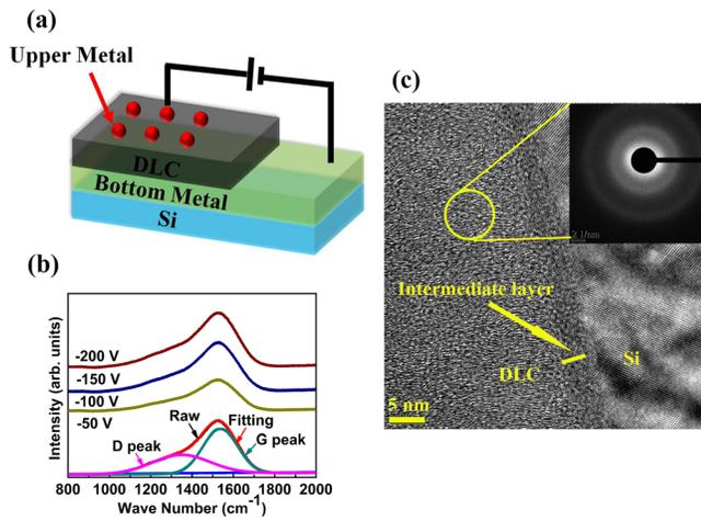
FIG. 1. The schematic diagram of the MSM structure (a), typical Raman spectra of the DLC (b), the cross-sectional HRTEM image, corresponding SAED pattern of the representative DLC deposited at  $-100$  V (c).
