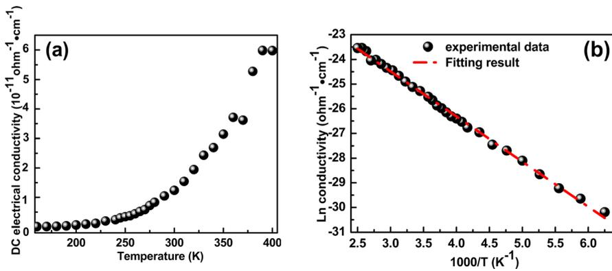
FIG. 3. The relationship between conductivity and the temperature (a), and the relationship between  $\ln(\sigma)$  and  $1000/T$  of the DLC film deposited at  $-50$  V (b). In Fig. 3(b), the black solid dots were experimental data and the red line was the fitting result according to the Arrhenius law.
