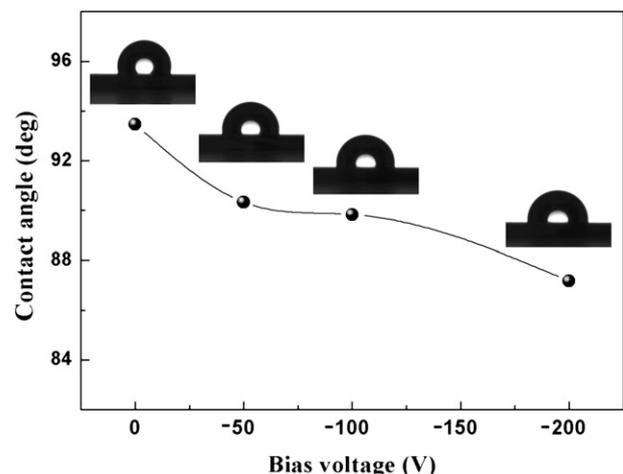
Fig. 8. Water contact angle of the films deposited at different bias voltage.
