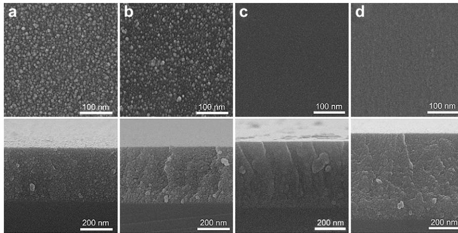
Fig. 7. Plan-view and cross-sectional SEM images of the films deposited at the bias voltage of (a) 0 V, (b) –50 V, (c) –100 V, and (d) –200 V.
