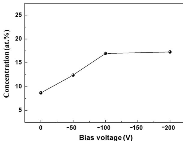
Fig. 3. Cr concentration of the films deposited at different bias voltage.
