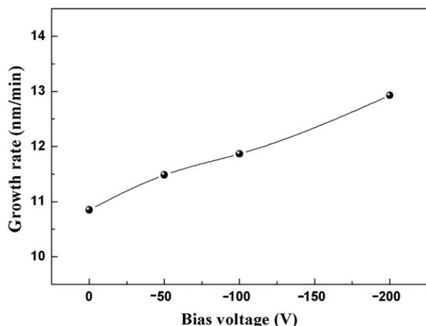
Fig. 2. Growth rate of the films as a function of the bias voltage.
