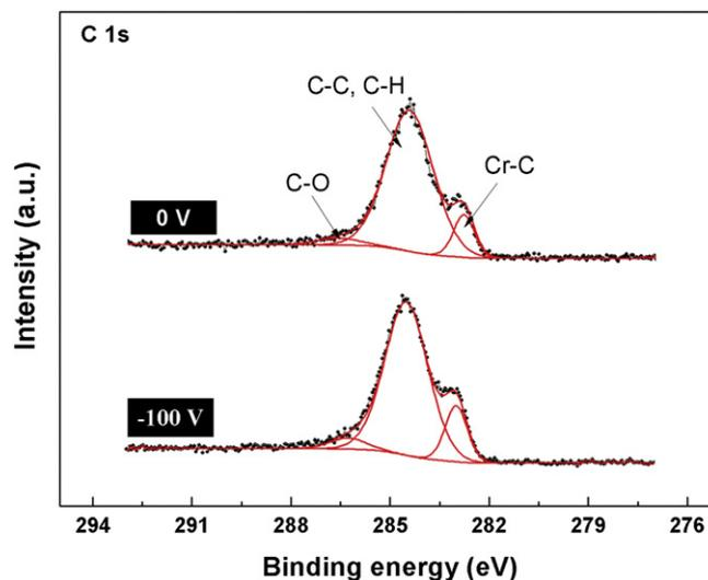
Fig. 4. Typical C 1s high-resolution XPS spectra of the films deposited with bias voltage of 0 V and  $-100$  V.
