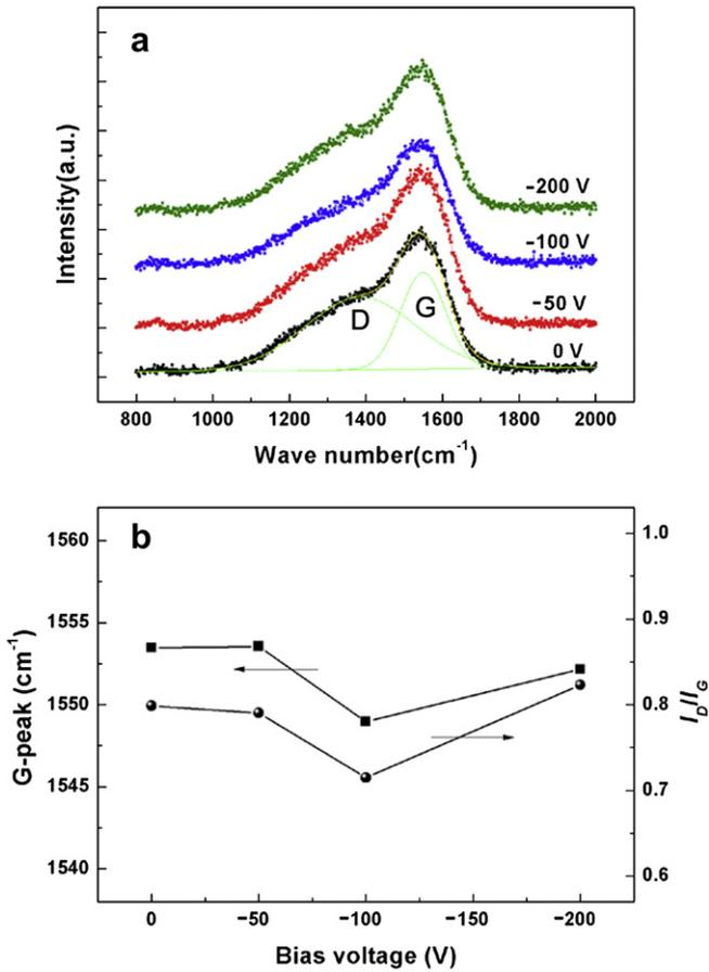
Fig. 5. (a) Typical Raman spectrum and Gaussian fitting, and (b) corresponding G-peak position and  $I_D/I_G$  of the films deposited at different bias voltage.
