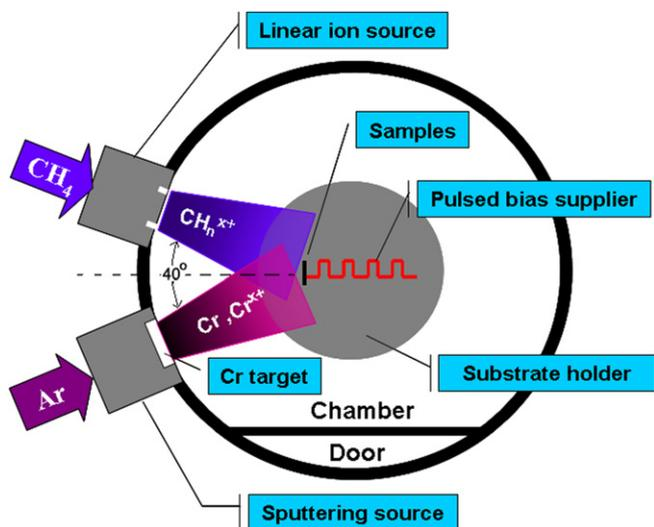
Fig. 1. Schematic diagram of the co-deposition system.
