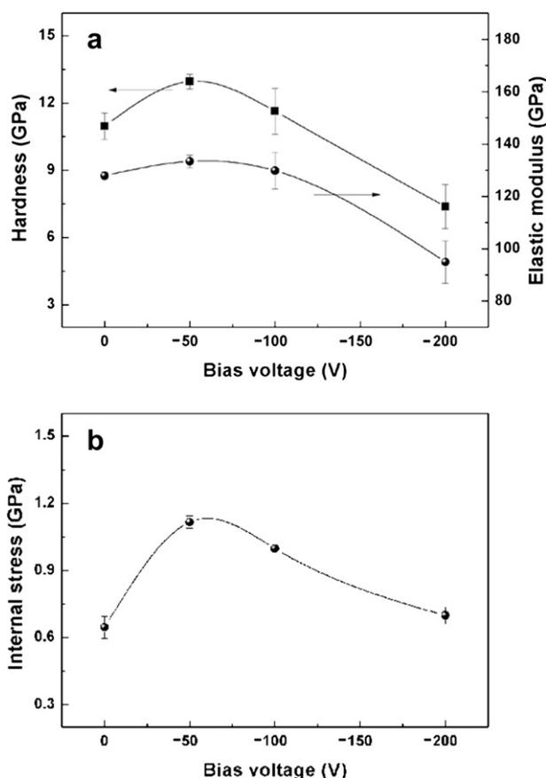
Fig. 9. (a) Hardness and elastic modulus, and (b) internal stress of the films as a function of bias voltage.
