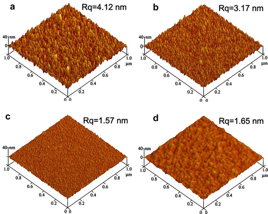
Fig. 6. AFM images of the films deposited at the bias voltage of (a) 0 V, (b) -50 V, (c) -100 V, and (d) -200 V.
