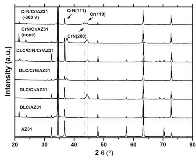
Fig. 1. XRD patterns of all samples prepared in this study.
