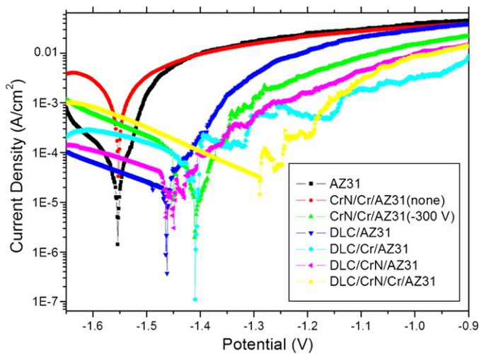
Fig. 4. Polarization curves of all samples prepared in this study.
