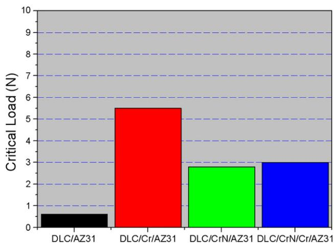
Fig. 3. Critical loads of the coated samples in the scratch test.
