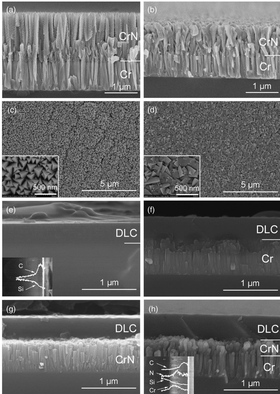
**Fig. 2.** Cross section and surface morphologies of all coatings prepared in this study: (a) and (c) CrN/Cr, no bias voltage applied, (b) and (d) CrN/Cr, bias voltage of  $-300$  V, (e) DLC, (f) DLC/Cr, (g) DLC/CrN, and (h) DLC/CrN/Cr.
